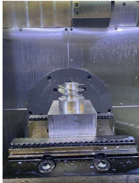
5-axis machining of a Kerosene inducer on a UMC 5-axis
