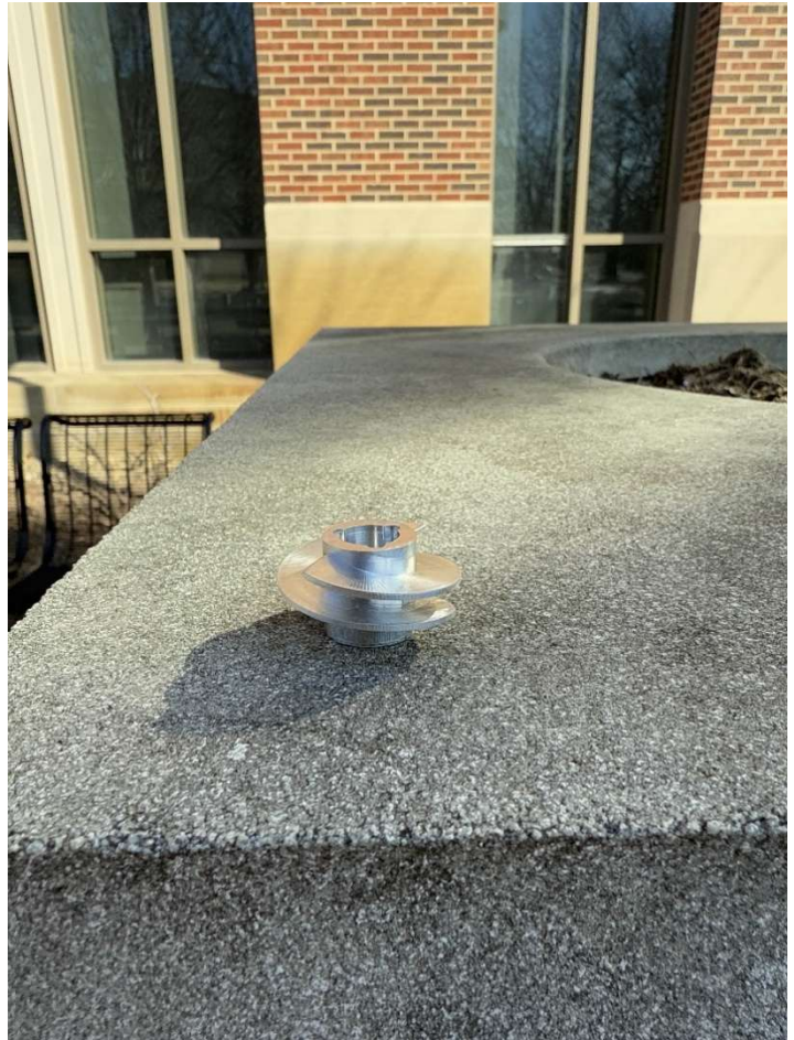
Final product: Kerosene Inducer for a turbopump
